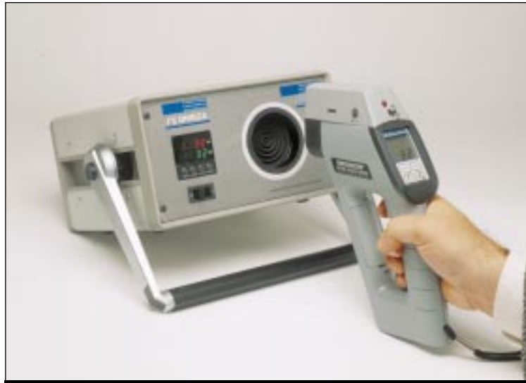
A handheld IR thermometer is calibrated against a commercial blackbody source—the internal cavity is designed to closely approach a blackbody's unity emissivity.
